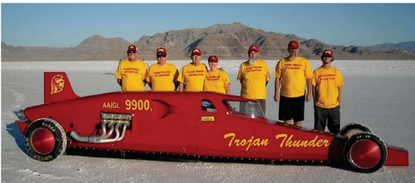
Stan Settles and his wife (center) are pictured with the technical team and the Trojan Thunder, ready to race on the Bonneville Salt Flats. Maximum speed over a measured mile was 263 miles per hour. The car is powered by a 565-cubic-inch unblown V8 gasoline engine, which generates more than 1,000 horsepower.
